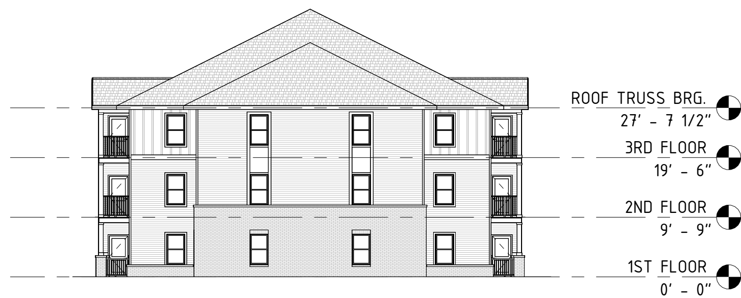
5 LEFT ELEVATION - BUILDING #1 1/16" = 1'-0"
