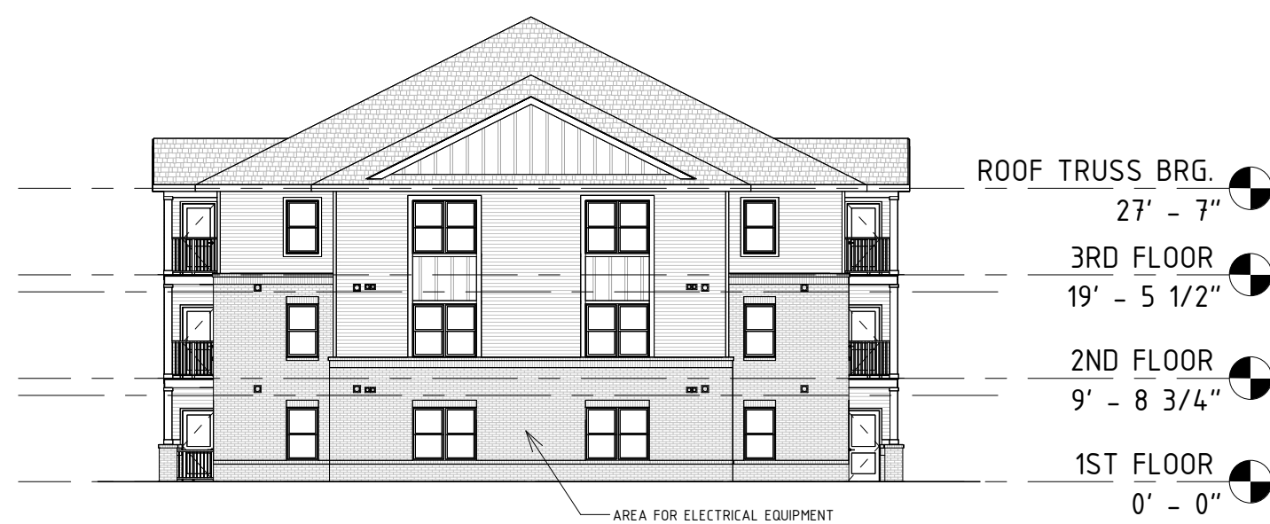
⑤ LEFT ELEVATION (SECONDARY) - BUILDING TYPE III (#1) 1/16" = 1'-0"
