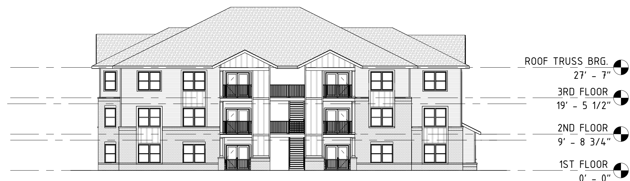
3 FRONT ELEVATION (PRIMARY - PARKING) - BUILDING TYPE I (#2 & #3) 1/16" = 1'-0"
