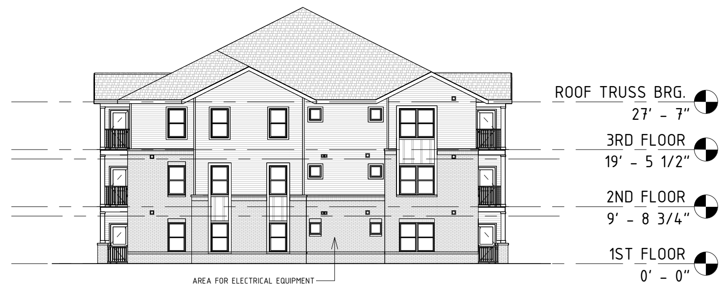
⑤ LEFT ELEVATION (SECONDARY) - BUILDING TYPE II (#4) 1/16" = 1'-0"
