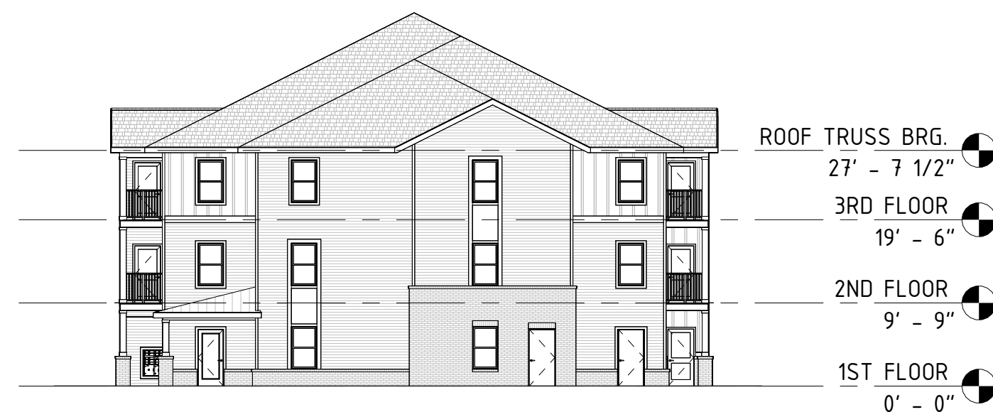
4 RIGHT ELEVATION - BUILDING #2 1/16" = 1'-0"
