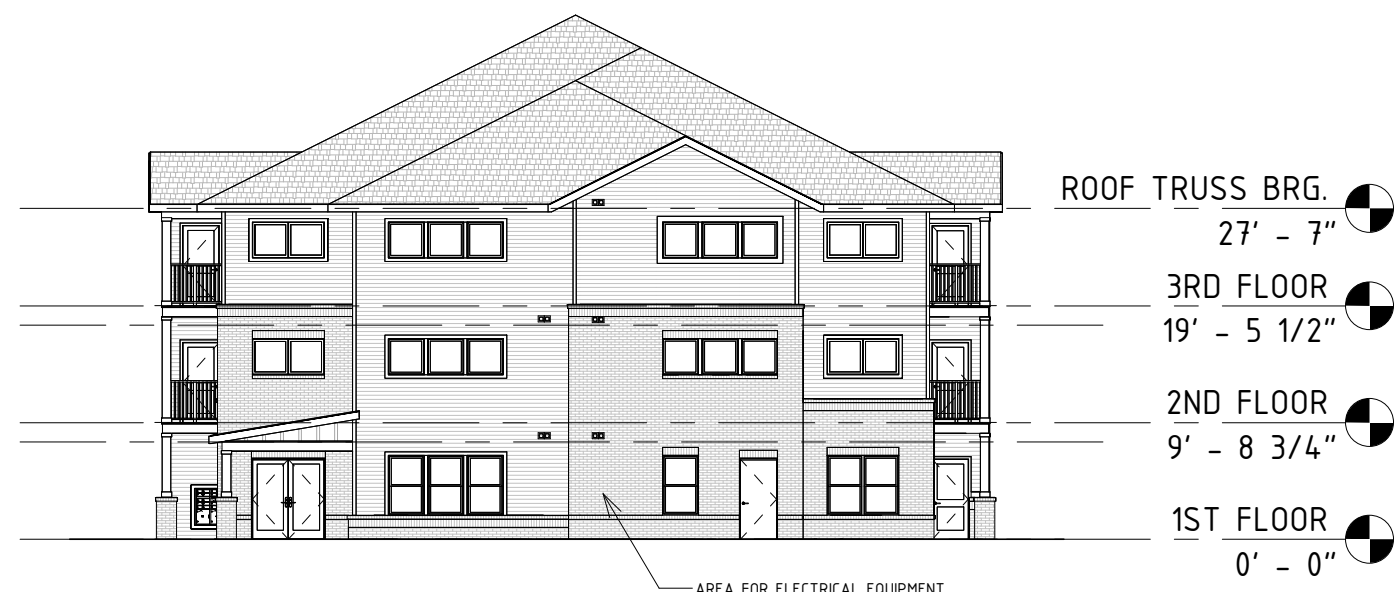
④ RIGHT ELEVATION (SECONDARY) - BUILDING TYPE III (#1) 1/16" = 1'-0"
