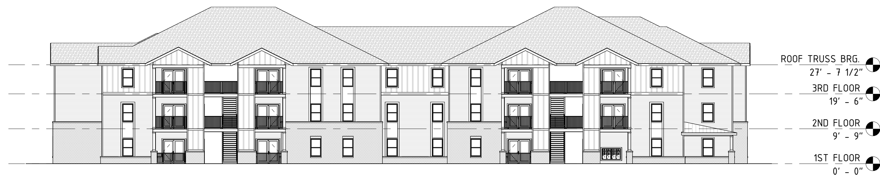
3 FRONT ELEVATION - BUILDING #2 1/16" = 1'-0"
