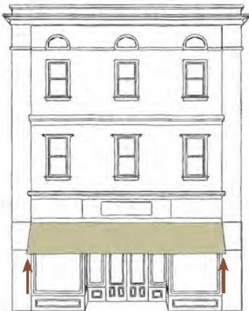
Acceptable awning placement
